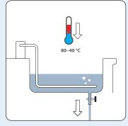
5. After the solution has cooled down (approx. 80-40'C) drain it\*\* and if necessary clean any remaining stains manually by using a cleaning pad or pot sponge. Areas around the deep fryer can be cleaned with PURINA fat solvent.
