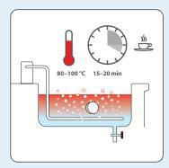
4. Heat up the deep fryer by using the boiling program\* to a temperature of 80-100' C for 15-20 minutes. For heavy stains the time can be increased or the dosage can be doubled.
